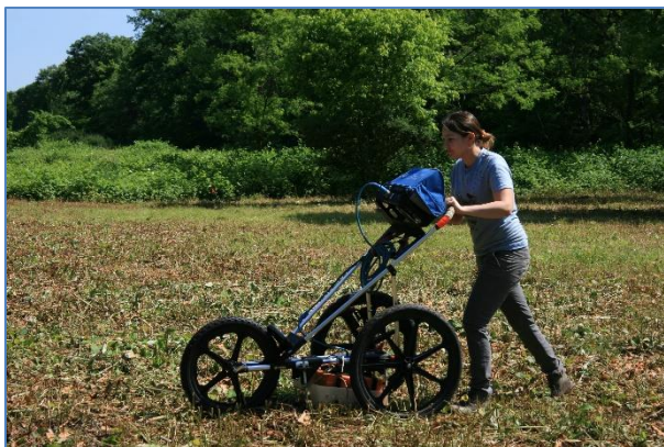
Using ground penetrating radar at the 2016 IUP archaeological field school.
