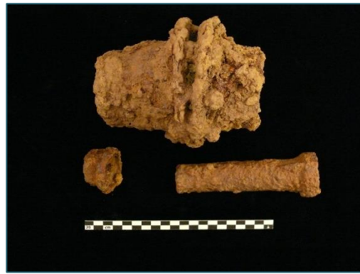
Wagon or carriage wheel parts including a wheel hub (top), a skein (bottom right), and a threaded end cap (bottom left) recovered from the site.
