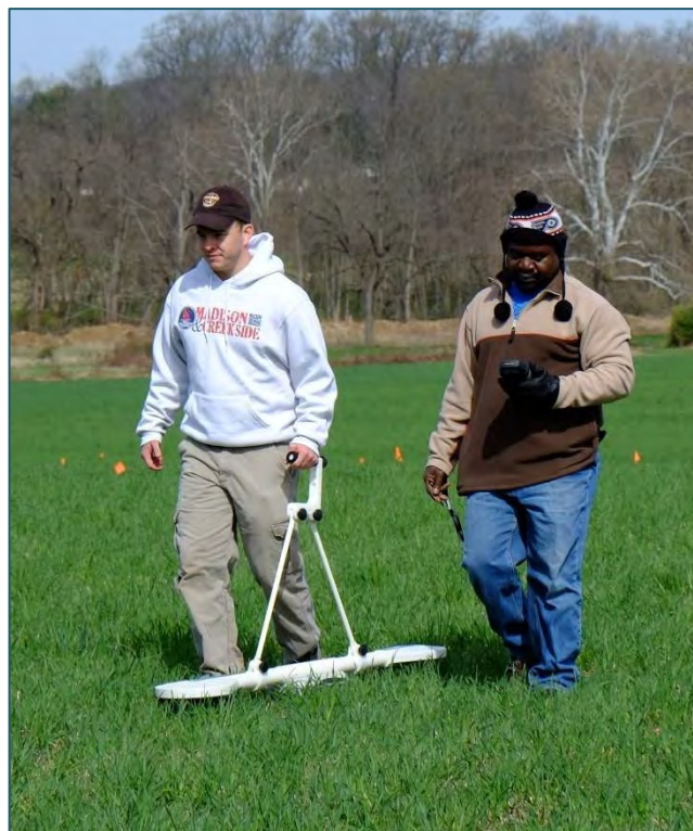
Dr. Joseph Zume (right) and Jake Percy collect data in the Wiest Farm block using a GSSI EMP Profiler unit. Photo courtesy of Dr. Paul Marr.
