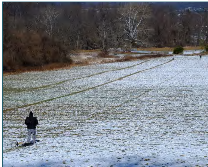
Dr. Sean Cornell pulls a Mala Geosciences X3M GPR control system with a 500 Mhz shielded antenna across a snow-covered field in the Schultz Farm block. Photo courtesy of Dr. Paul Marr.
